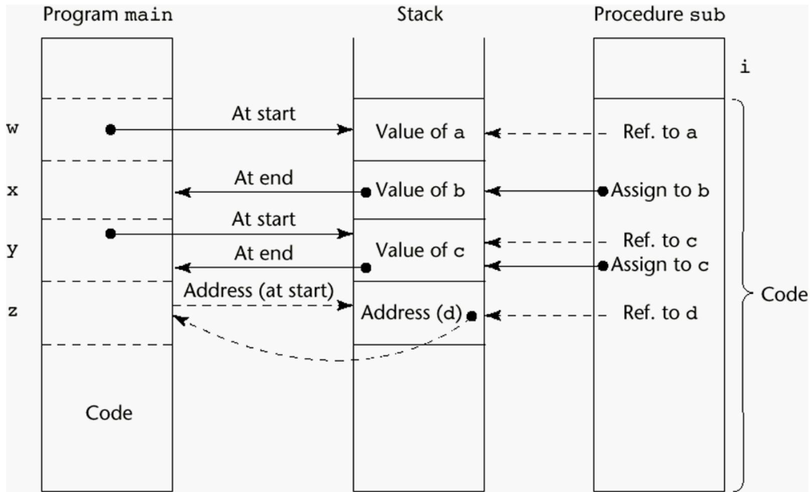
Main program calls `sub(w,x,y,z)` where **w** is passed by value, **x** is passed by result, **y** is passed by value-result, and **z** is passed by reference
