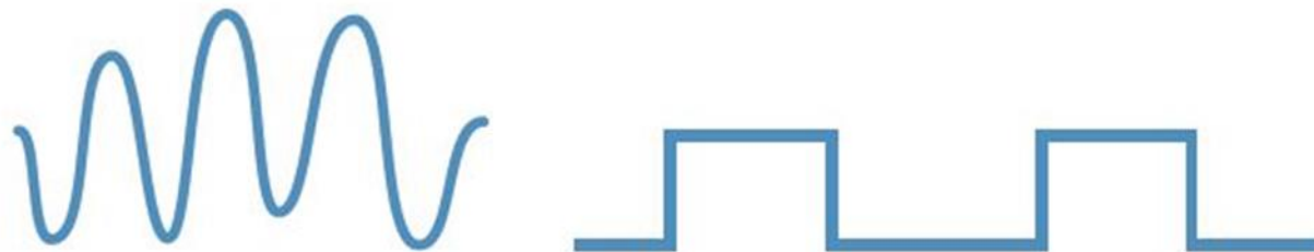
FIGURE 3.2 An analog signal and a digital signal
