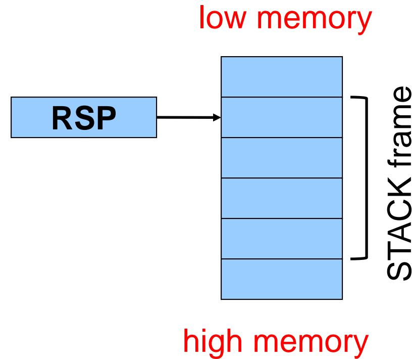
Allows use of the STACK section of memory, and special-purpose stack manipulation instructions
